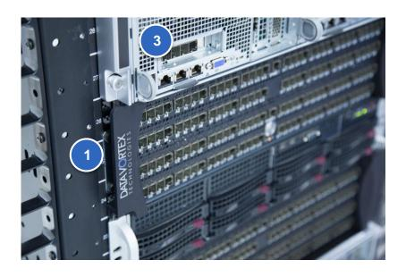
The DV208 is an advanced computing system with an integrated interconnect and software technology that actually embraces processor-to-processor communication. Each system contains the revolutionary, patent-protected Data Vortex interconnect technologies: the Data Vortex Switch Boxes and the Vortex Interface Controllers (VICs).
